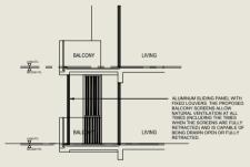
TYPICAL RETRACTABLE BALCONY SCREEN - SECTION A-A
