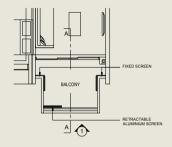
TYPICAL RETRACTABLE BALCONY SCREEN (FULLY RETRACTED) - PLAN
