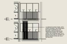
TYPICAL RETRACTABLE BALCONY SCREEN(OPEN) - ELEVATION 1
